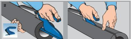
The use of the cutter is illustrated in these two diagrams. Let the blade run along the tube without the tool's surfaces touching it to get a neat, clean cut.
